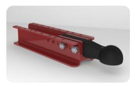
The sprayer needs to be equipped with a ball coupling which fits the K80
