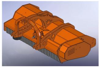
This machine has been specialally designed for heavy wood such as cherry wood which can not easily be shredded. This is achieved by the high speed and large diameter of the rotor which ensures a high circumferential speed of 54 m/s (1000 rpm)
