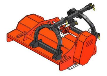
This machine has been specially designed for heavy wood such as cherry wood which van not easily be shredded. This is achieved by the high speed and large diameter of the rotor which ensures a high a circumferential speed of 54 m/s (1000 rpm)
