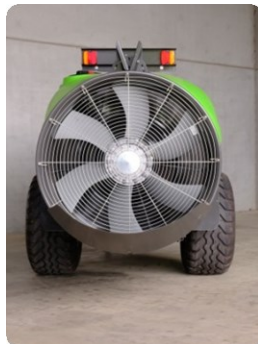
pic: 3 propellor ø 900 mm
