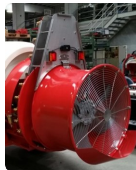
pic: 4 propellor ø 900 mm with A-frame
